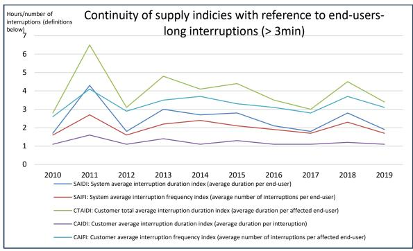
Figure 1 Continuity of supply indices with reference to end users - long interruptions.
