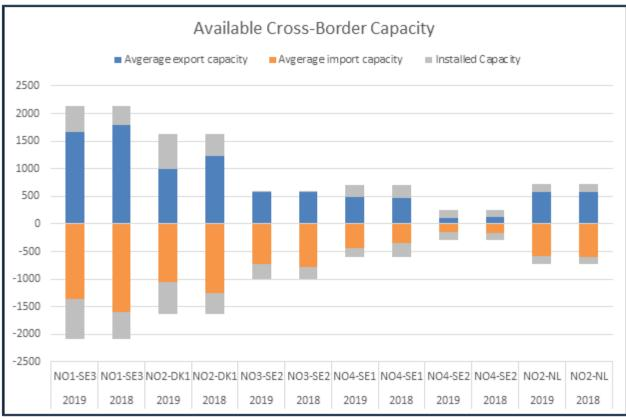
Figure 5. Available capacity in 2019 and 2018 for export and import as a portion of installed capacity for each cross-border interconnector. Source: Nord Pool Spot and SKM Syspower.
