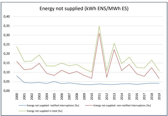
Figure 3 Energy not supplied (ENS) in thousand relative to the energy supplied (ES) to end users in Norway since 2000.
