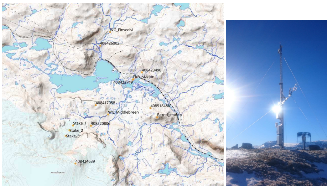
Figure 9 High resolution measurement infrastructure at Finse alpine research station, including a Flux tower (LATICE Flux), two discharge stations, seven WSN (wireless sensor network for hydrometeorological data) and ablation stakes for snow (installed fall 2016).
