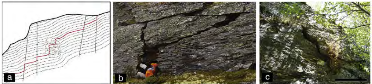
Figure 17. A complex basal failure surface as proposed by Bøhme et al. (2013). (a) A schematic profile indicating that the failure surface follows foliation in some parts, but steps down along pre-existing joints or fold hinges. (b) and (c) Step-path failures observed in smaller scale in the field.
