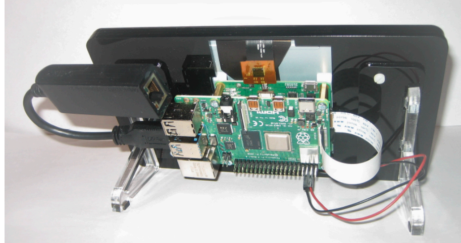
Figure 5: Raspberry Pi IED with Touch HMI and Gbit Ethernet Interface
