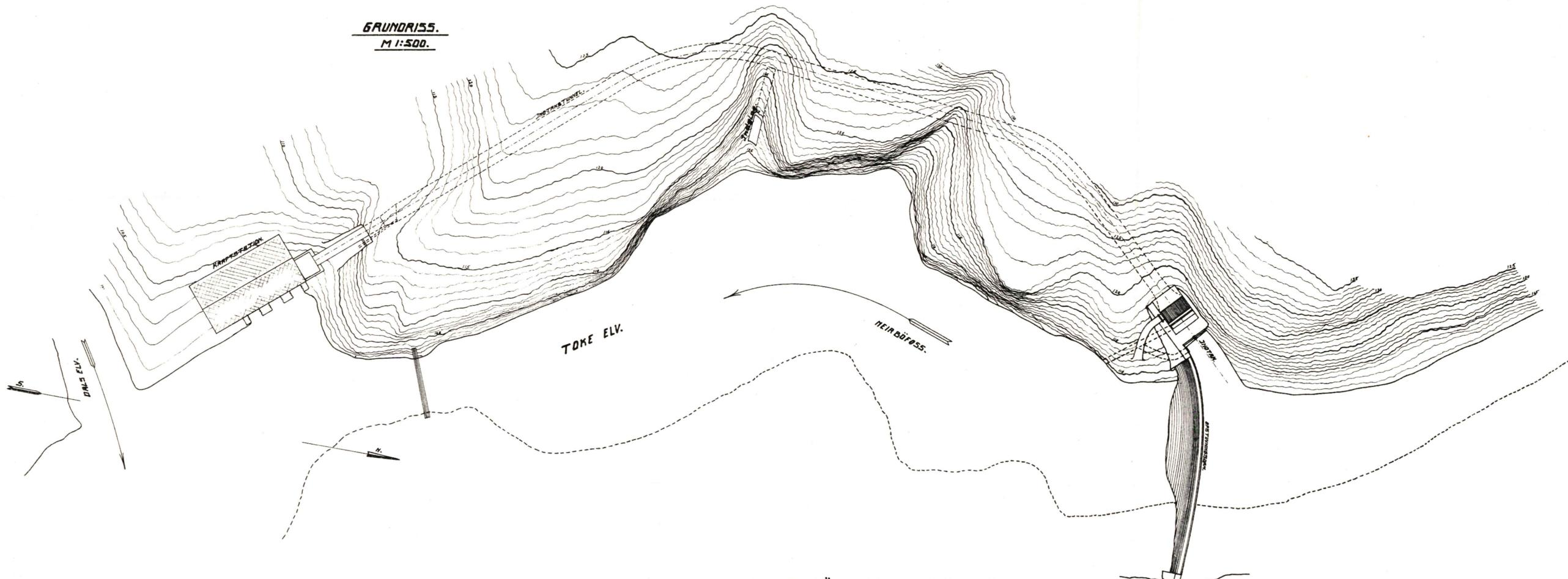
LÆNGDEPROFIL AV INOTAK, TUNNEL, RØRLEDNING OG KRAFTSTATION.
