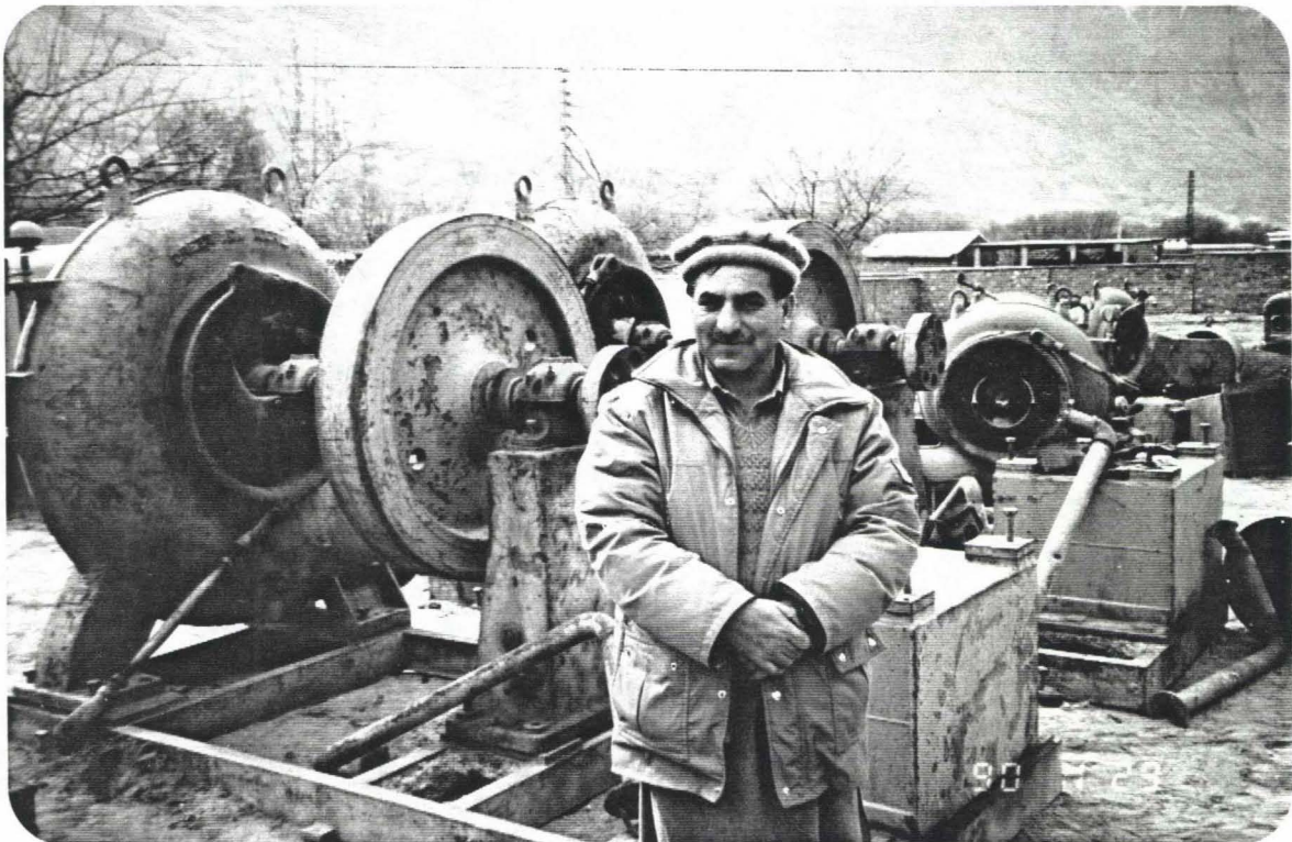
OLD TURBINES FROM KARGAH CAN BE REFURBISHED IN THE PLANNED WORKSHOP AND USED IN SCHEMES AS DANYOR PH.2
