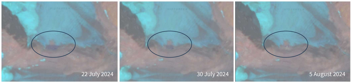
Figure 13-9 Sentinel-2 images of the glacier lake at Midtbreen from 22 July (left), 30 July (middle) and 5 August (right) 2024. The images show less water in the lake on 30 July than it was on 22 July and empty lake on 5 August, indicating that the lake was drained at the turn of the month between July and August. Source: Varsom Xgeo.
