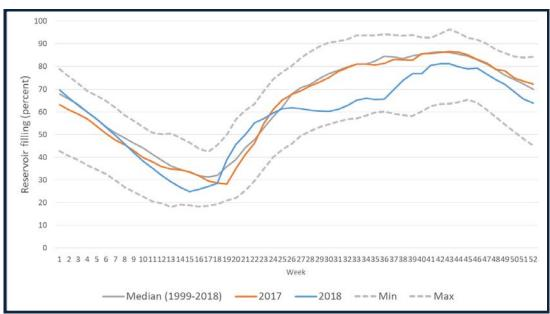
Figure 7. Hydro reservoir levels in Norway. 100 percent represents 84 TWh storage capacity. Source: NVE
