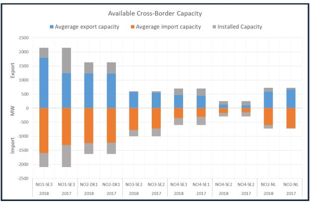
Figure 5. Available capacity in 2018 and 2017 for export and import as a portion of installed capacity for each cross-border interconnector. Source: Nord Pool Spot and SKM Syspower.
