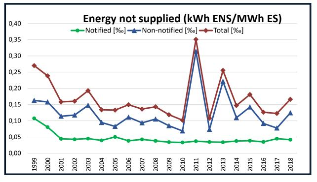
Figure 3. Energy not supplied (ENS) in per thousand relative to the energy supplied (ES) to end users in Norway since 1999.
