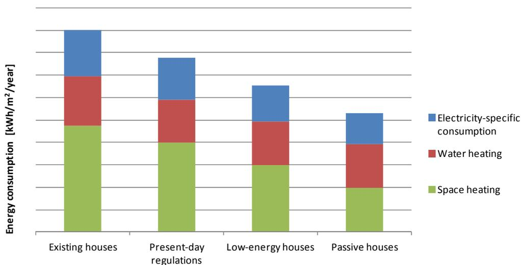
Figure 3.15 Typical energy consumption by end-use for houses built to different technical regulations
