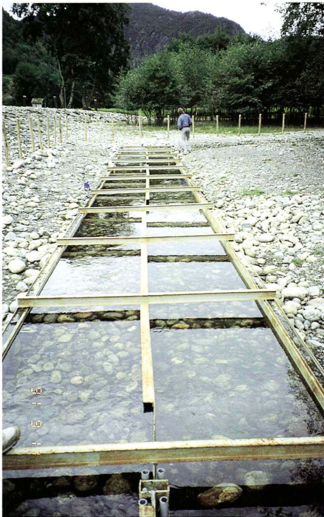
Experimental channel in the Suldalslågen, September 1991. Grain was added to the left side, while the right side was a control zone (photo: Jon Arne Eie).
