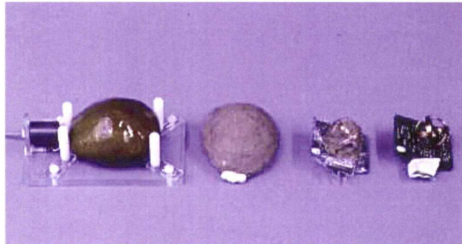
Figure 3: Logging pebble components, illustrating from R-L, Circuitry and receiving coils, encapsulated circuitry, data download jig.
