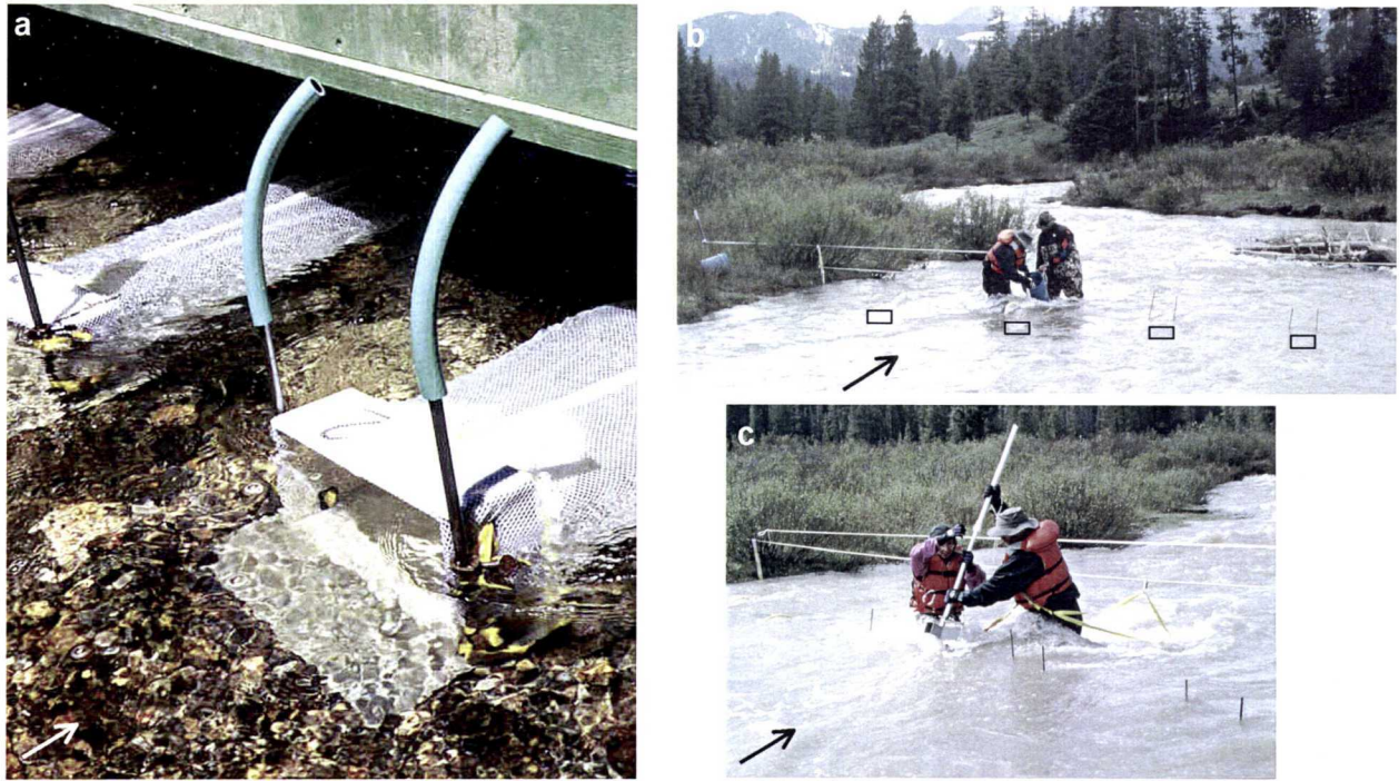
Fig. 2 Bedload traps with ground plates at East St. Louis Creek in low flow (a); Emptying bedload traps at Little Granite Creek in bankfull flow. The open squares indicate the positions of 4 of the 6 bedload traps which are completely submerged by flow (b). Using a 3-inch Helley-Smith sampler at Little Granite Creek in bankfull flow (c). Arrows indicate flow direction.
