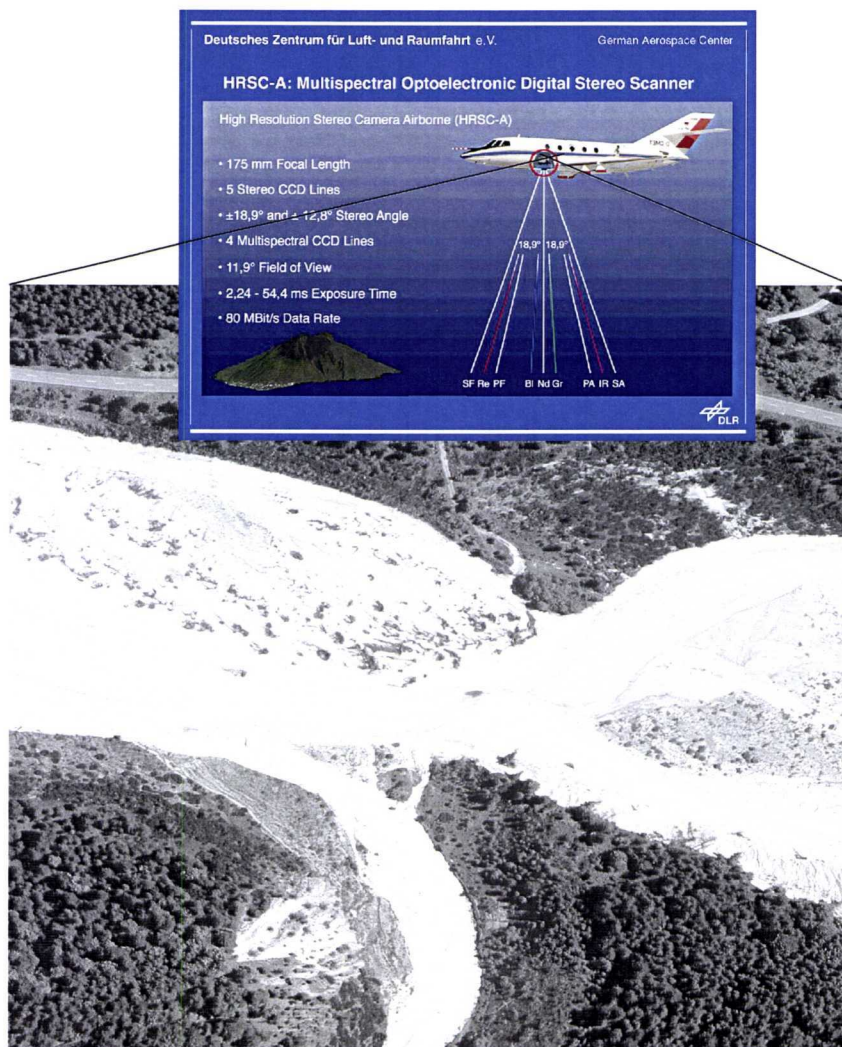
Fig. 4 Detailed analysis of sediment size, arrangement and volume changes of river beds based on HRSC image analysis with a grid size of 17.5 cm.
